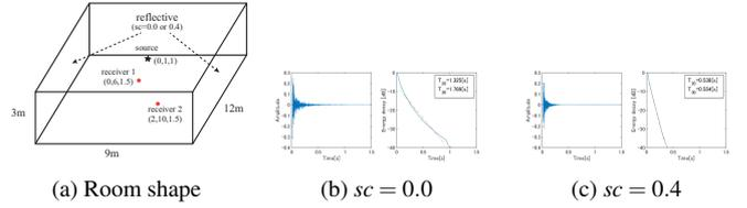
Figure 1. Room shape and impulse responses and energy decay curves.
